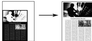
When selected a true Bi-Mode sensing allows the Z-Scan 47 to automatically determine the film type so you get a positive printout whether you are using negative or positive film.
