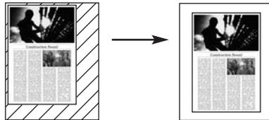
The system generates an image that is centered on the printed page, from an image on the screen with a masked frame.
