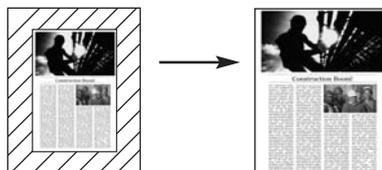
Fits the image on the screen onto the entire surface of the print (50% to 200%).
