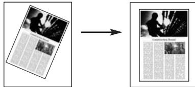
The machine automatically corrects any skew of up to 30 degrees when the image is printed.
